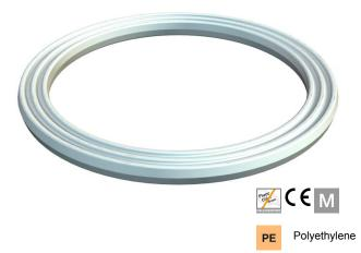
Connection thread sealing ring, suitable for all plastic cable glands, with metric thread according to DIN EN 60423 or ISO 68. The internal diameters of the sealing rings are designed in such a way that they can be pre-mounted in a captive manner.
