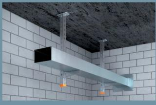
Suspended mounting on mounting system
